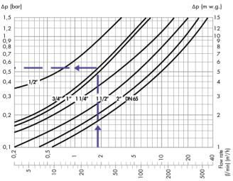
Reference conditions: Upstream pressure = 8 bar Downstream pressure = 3 bar
