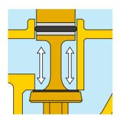
In the figure, the thrust towards the opening is counterbalanced by the force created by the closing pressure acting on the compensating piston. Since the piston has a surface area equal to that of the obturator, the two forces cancel each other out.
