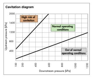
In order to minimise the risk of cavitation in the reducing valve, which could cause malfunctions with the risk of erosion in the seal area, vibration and noise, you are strongly advised to refer to the operating conditions specified in the diagram.
